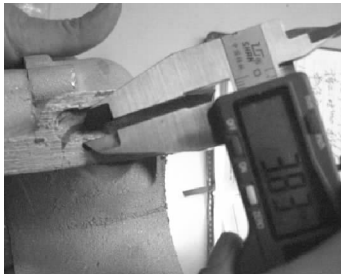
图9 测量缺陷实际尺寸 Fig.9 Actual dimension of measured defects
