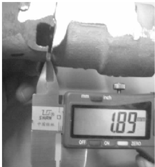
图 13 目视测量缺陷尺寸 Fig.13 Visual measurement of defect dimension
